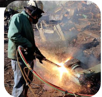
50 lbs. of iron powder provides 8 hours of cutting on avg.
