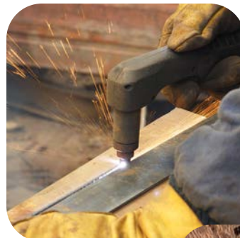
Electric plasma cuts metal up to 2" thick
