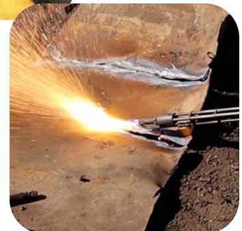
Iron powder cuts metal up to 36" thick
