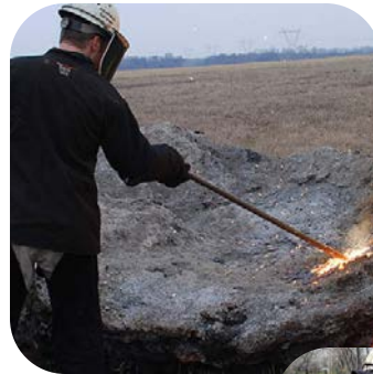
Burning bars require constant swapping over 8 hours
